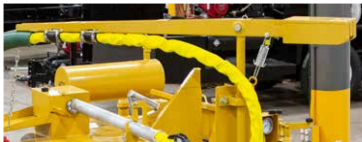
Ergonomic counter balanced hose boom
