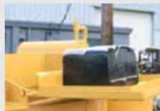
Anti-Splash Material Loading Hatch
