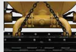
Dual Easy-Open Butterfly Sealer Discharge Valves
