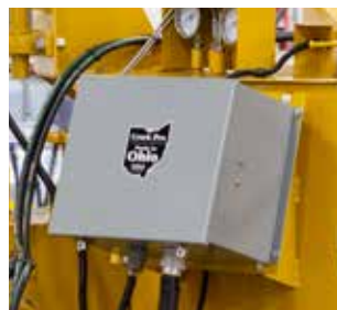
Steel enclosure for the control box
