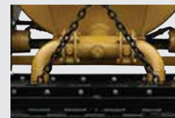
Dual Easy-Open Butterfly Sealer Discharge Valves
